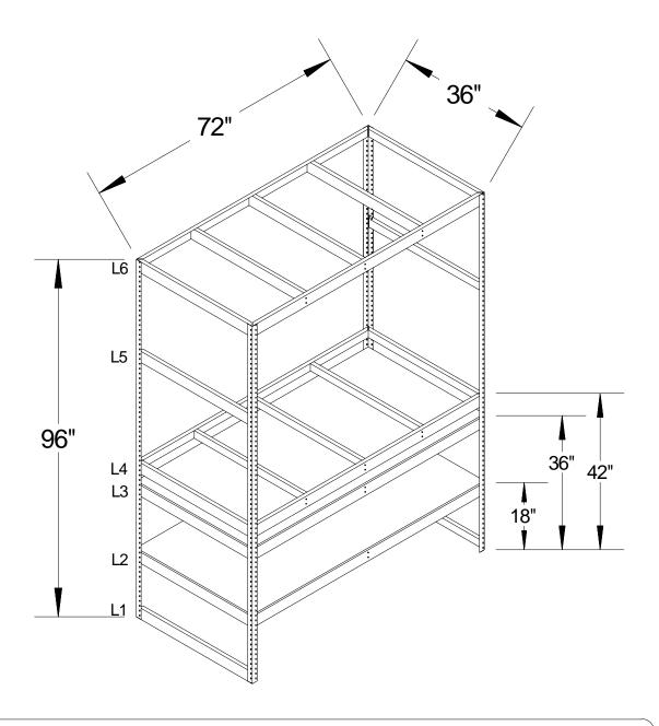
MODEL #3350 MUFFLE & PIPE STORAGE RACK READ RIVET RACK BASIC ASSEMBLY INSTRUCTIONS BEFORE ASSEMBLING
